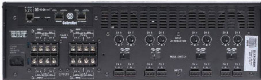
CTs 8200USP/CN Back Panel (note USP/CN CobraNet™ module at top)
